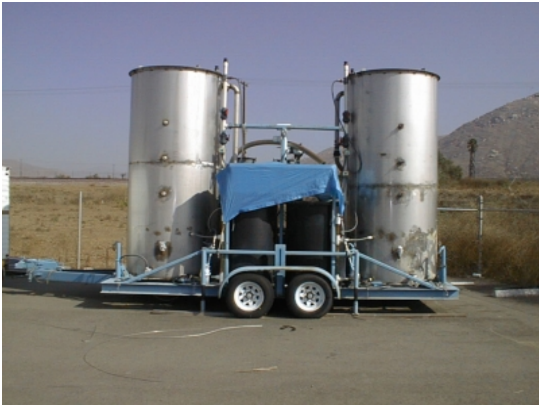
Figure 3.2 Picture of the pilot biotrickling filter. The air flows in series through the two tanks.
