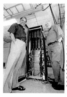
Bourns' ALTIX 4700 SUPERCOMPUTER CAN BOOST HIGH-END COMPUTING AND DATA ANALYSIS BY UP TO 1,000 TIMES ONE OF THE LARGEST SINGLE ALTIX 4700s IN THE University of California SYSTEM. WITH ITS 64 INTEL TANIUM 2 PROCESSOR CORES AND FEATURES 128 GB OF SYSTEM MEMORY, IT HAS ALREADY BEEN INVALUABLE IN BOURNS RESEARCH ON RECONFIGURABLE PROCESSORS. BIOINFORMATICS RESEARCH. COMPUTER ARCHITECTURE AND OTHER RESEARCH. IT IS ALSO USED AS A CLASSROOM TOOL IN COMPUTER ARCHITECTURE CLASSES.
