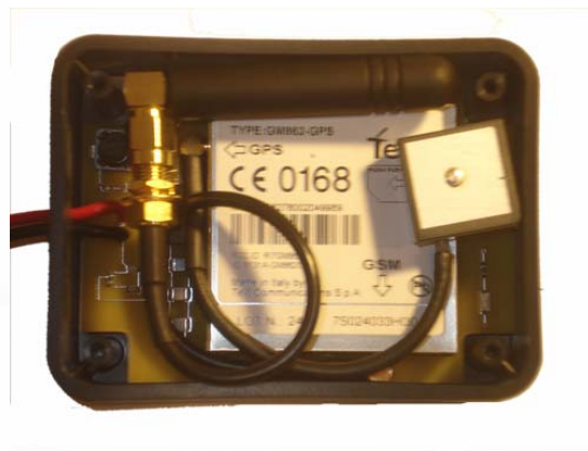
AVL (PCB, Enclosure, Antennas)
